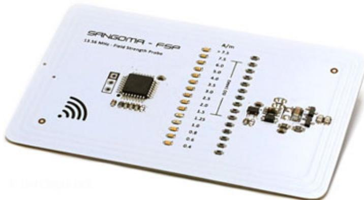
Our RFID/NFC field strength probe measures the strength of the emitted field and displays this on a graded and labelled 15 step three colour LED indicator. The probe is sized exactly as a standard ID1 card (86mm x 54mm) and has an etched antenna that reflects a typical contactless or dual-interface smartcard or NFC tag. It can be used to obtain a good measure of a reader's performance at different distances and positions, and to get an indication of the actual field strength in A/m.
